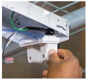
**3.** Break apart the 1-piece mounting bracket kit into 3 individual pieces. Install a small bracket to each end of the fixture and the large bracket at the center of fixture (for 8' fixtures only) by bending them over the fixture to fit the exact width and fastening them to the fixture with the provided tek screws.
