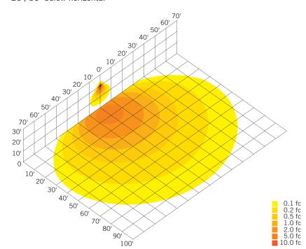
Ground mounted at 6" above ground, 10° above horizontal, shining towards building exterior wall at 281 away.
